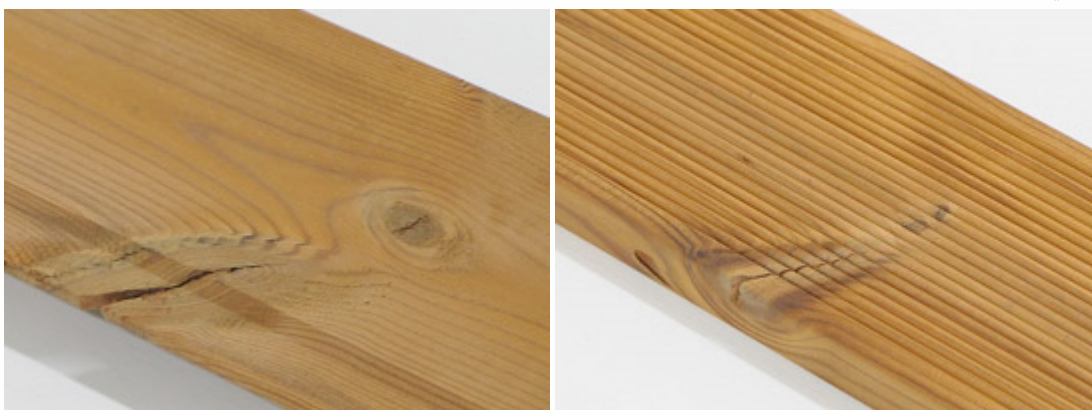
SINGLE CRACK OF A KNOT
