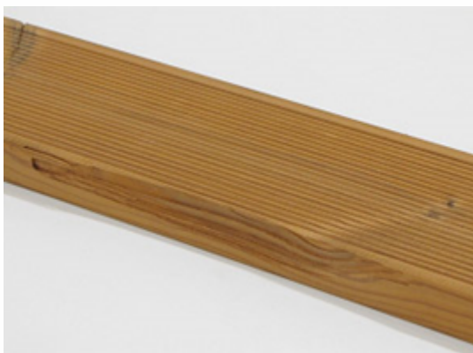
SEVERELY DEFECTED EDGES
